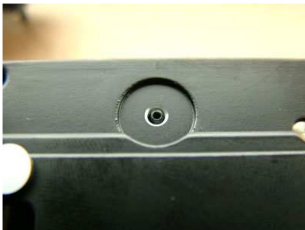
Here is a filter that cleans the air entering the drive. A drive isn't airtight, instead it allows the pressure to be equalized in the drive but the air coming into the drive has to be clean.
